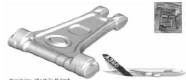
图5 A380 飞机 Ti-10V-2Fe-3Al 起落架壁板 (俄罗斯, 750 MN 水压机模锻) Figure 5 Ti-10V-2Fe-3Al under carriage wall panel of A380 airplane (Russia, 750 MN hydraulic press die forging)
